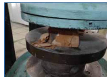
Testing the brick at IIT lab
