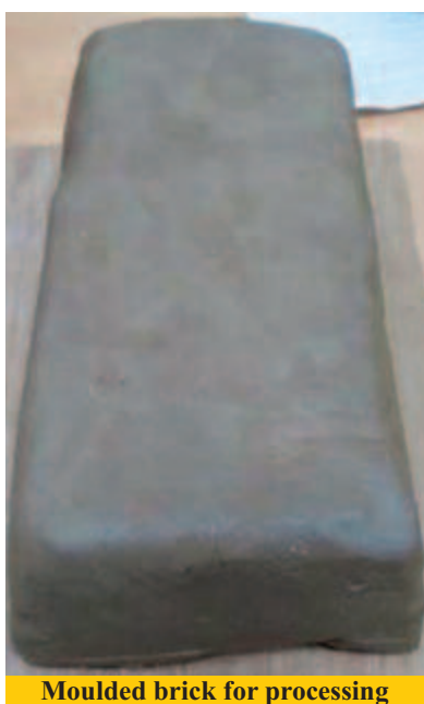
Front view of eco-brick prototype made by the team using fly-ash, coco-fibre, rice husk and plastic shreds
