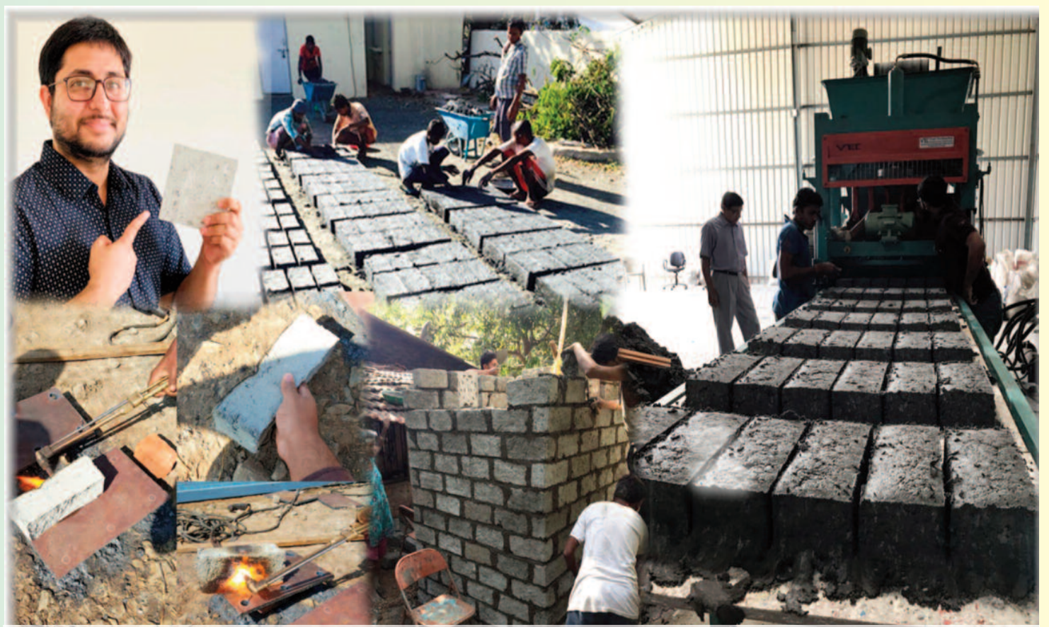
Dr Binish Desai and the innovative bricks made from recycled plastic waste during the pandemic
